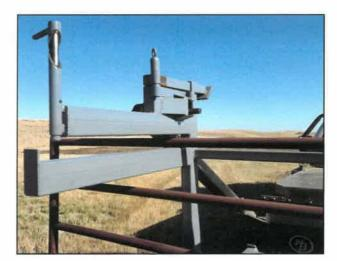
♦ Utilizing your bed arms you can hover the Panel Pal inches above the ground making loading and unloading much easier, especially with one person.
