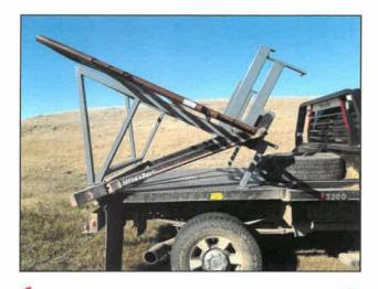
◆ Retractable legs can keep the panels far enough off the bed to see under with the mirrors and go over most gate posts.
