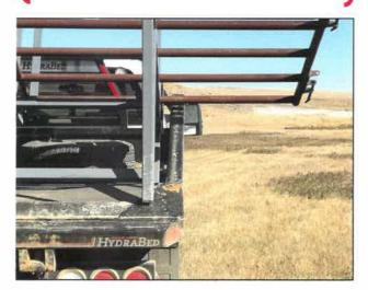
◆ An adjustable fork in the middle allows you to carry panels off to one side somewhat and yet keeps them from sliding back and forth when the panels' upright is put in it.
