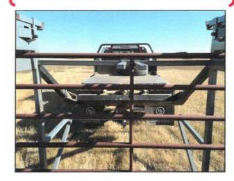
◆ Retaining latches can remain open while loading or unloading panels. Then when ready to transport, the latches are put into the closed position, keeping the panels secure.
